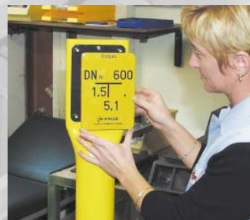
Marker plate fitted at FP and inserts fitted to your specifications
