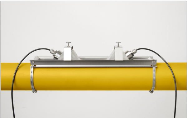
Metallic mounting rail with transducers
